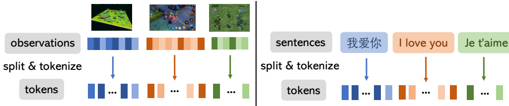
Figure 3: Games as Languages. (Left) Tokenize different observations from different games. (Right) Tokenize different sentences from different languages.
