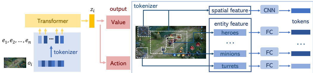
Figure 2: (Left) Overall framework of MAGENTA. (Right) An example tokenizer for HoK. Spatial features are as images and entity features as vectors.
