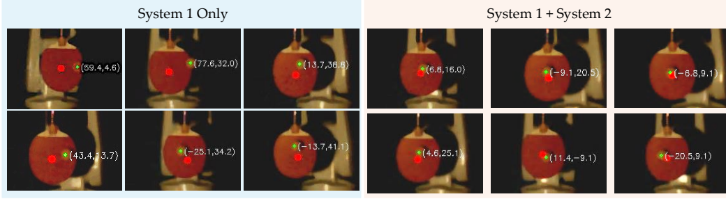
Figure 4: Visualization of ball-racket contact precision with and without System 2. Spike-based camera images show the ball center (green) and racket center (red) at contact moment. The reduced offset with Fast-Slow System demonstrates improved ball interception accuracy.
