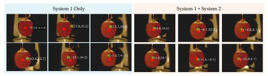
Figure 4: **Visualization of ball-racket contact precision with and without System 2.** Spike-based camera images show the ball center (green) and racket center (red) at contact moment. The reduced offset with Fast-Slow System demonstrates improved ball interception accuracy.
