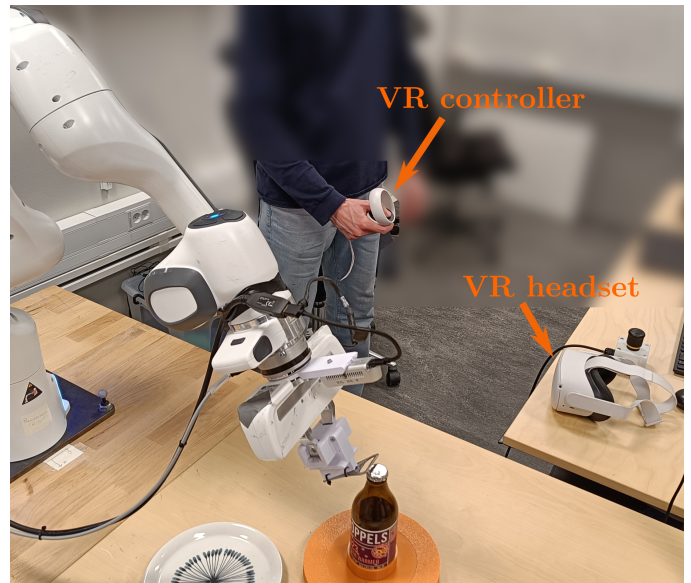
Figure 1: Example usage of the Quest2ROS teleoperation on a Franka Panda robot. The headset is placed on the table with an unobstructed view of the handheld controller, which in turn is used to teleoperate the robot.
