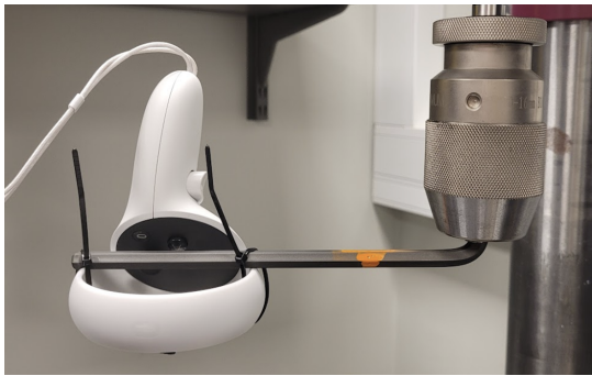
Figure 7: The figure shows the setup used to fix the controller to follow a circular path used for accuracy evaluation.
