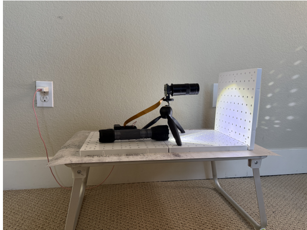
Figure 1: Custom imaging rig for textile microtexture analysis, featuring a Raspberry Pi HQ Camera mounted on a tripod, dual high-intensity flashlights for off-axis illumination, and a perforated panel used as a stand for clothing and sample backdrop.
