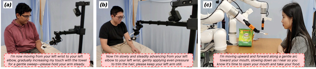
Figure 3: The three tasks implemented and used in the user study, along with example communications generated by CoRI: (a) simulated bathing —moving a piece of dry washcloth along the user’s forearm, (b) simulated shaving —moving a surgical clipper with a fake razor along the user’s forearm, and (c) feeding —bringing the user a spoonful of food.
