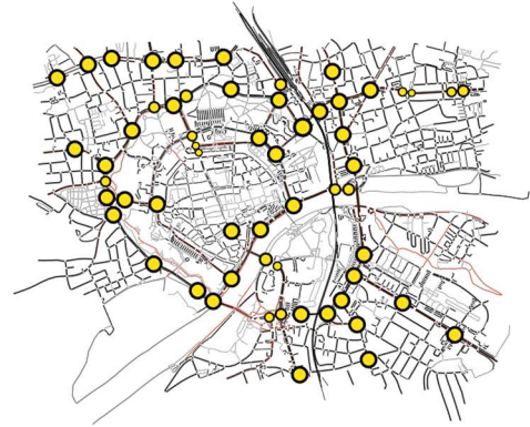
Fig. 2 Ingolstadt scenario network. Circular yellow markers indicate the position of traffic signal controls.
