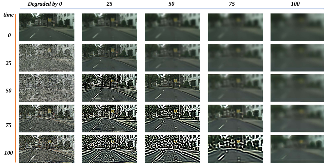
Figure 11: Examples of image deblurring, horizontal coordinate represents the level of image degradation, and vertical coordinate indicates the t used in the inference.
