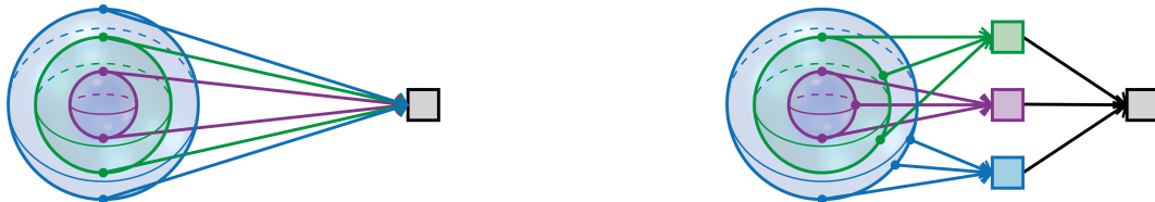
Figure 1: Visualization of the standard global pooling method (left) and our proposed Group-Invariant Global Pooling (right). Each sphere represents an orbit in SO(3) . GIGP builds group-invariant representations by aggregating each orbit separately, unlike global pooling. This leads to better-principled aggregation that is designed to respect the given symmetry.
