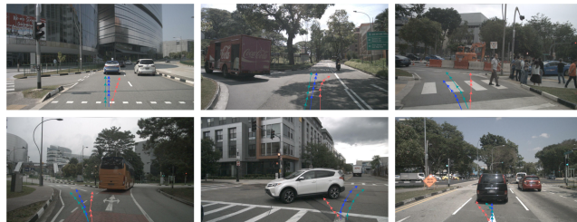
Figure 4: Qualitative comparison of waypoint predictions across diverse driving scenarios. Ground truth trajectories (blue), zero-shot model predictions (green), and fine-tuned model predictions (red) of Gemma in LORA way are overlaid on front-camera images. Zero-shot predictions closely track ground truth across all scenarios, while fine-tuning for decision-explaining systematically compromises geometric reasoning and trajectory planning capabilities.
