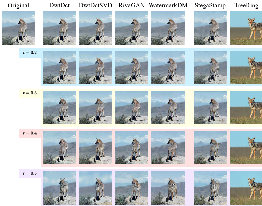
Figure 14: Watermarked Images subjected to the latent diffusion purification attack are shown with varying values of the parameter t . For t = 0.5 , the attack drastically changes the images in most cases (except for TreeRing).
