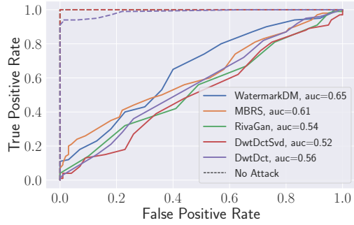
Figure 3: ROC curves for empirical robustness of image watermark methods against diffusion purification attack with t = 0.2 . The dashed lines show the ROC curves of methods without attacking them.
