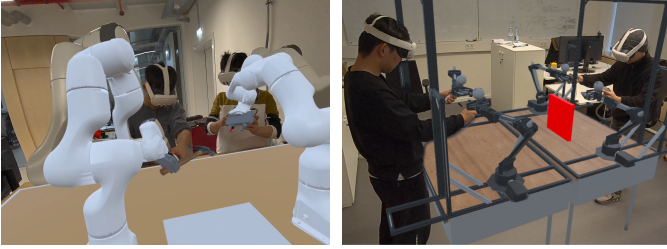
Fig. 6: Collaborative manipulation in the simulation via XR. The left image shows the collaborative manipulation for hand over a hammer between two Franka Panda robots by Kinesthetic Teaching, and the right image shows that collaborative manipulation for hand over a red board between two Aloha 2 Arms by Motion Controller.
