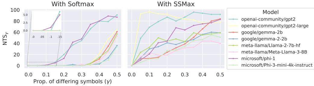
Figure 9: Next-token sensitivity of decoder-only language models to input perturbations. Each line shows the number of sample sequences (out of 100) that produce a different next-token than zero, as a function of the proportion of differing symbols. Left: Models with standard softmax in attention layers. Right: Models replaced with ssmax in attention layers.
