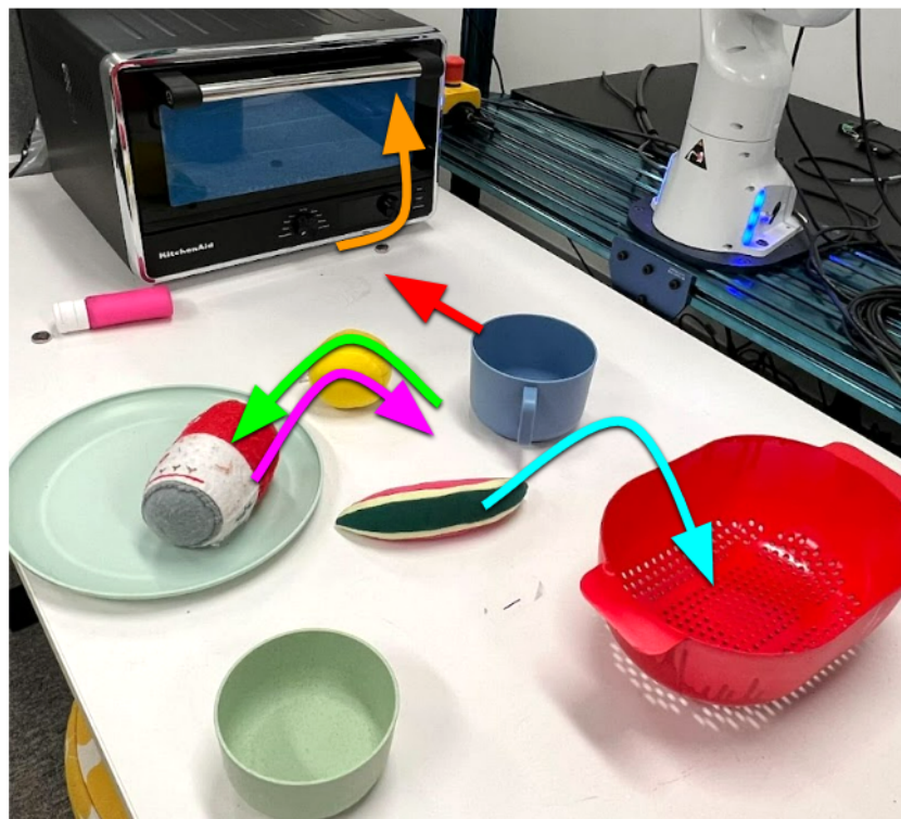
Figure 7: Real robot tasks. Illustration of the five real robot tasks, namely: drag mug, close toaster, place can on the plate, place can on the table, put watermelon in strainer. The colored arrows approximate the task trajectories.
