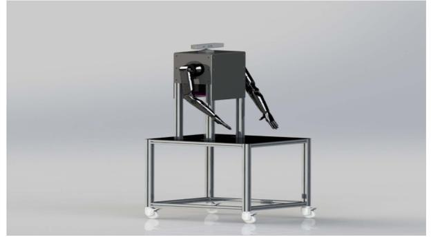
Fig. 4. Developed dual-arm robot for human-robot collaboration.
