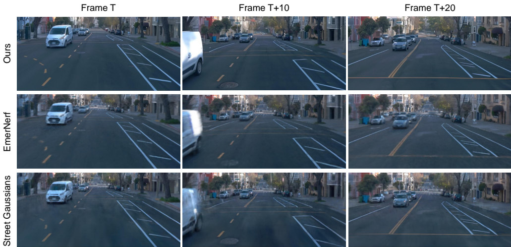
Figure A: Visualization comparison on moving objects. We compare the performance of NVS methods where moving objects are visible in camera views. In the shown case, our proposed method can generate more accurate images of vehicles driving in the opposite lane. Images are synthesized on training views.
