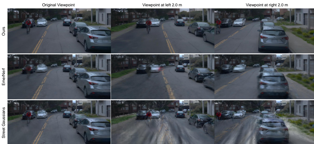
Figure 5: Visualization comparison on novel trajectories. We show the camera views synthesized by NVS methods on the original training viewpoint, viewpoint 2.0 m left of the original viewpoint, and viewpoint 2.0 m right of the original viewpoint.
