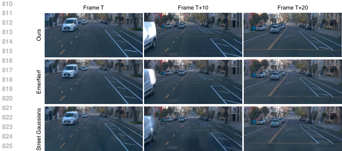
Figure A: Visualization comparison on moving objects. We compare the performance of NVS methods where moving objects are visible in camera views. In the shown case, our proposed method can generate more accurate images of vehicles driving in the opposite lane. Images are synthesized on training views.
