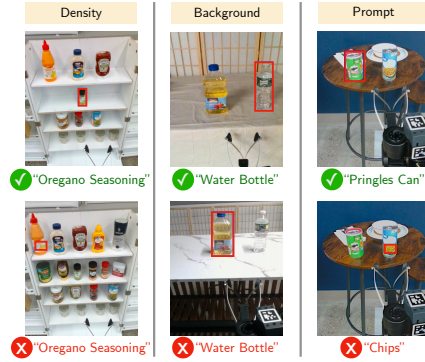
Figure 5: Vision backbone example failure cases. We find that a cluttered background and poor lighting conditions to lead to a sub-optimal set of bounding boxes for CLIP to score, while more specific prompts produce better bounding box proposals.
