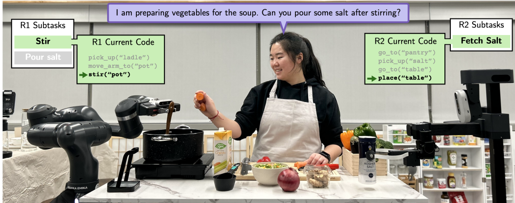
Figure 1: MOSAIC cooking in the kitchen. MOSAIC interacts with a user via natural language and controls a tabletop manipulator (R1) and a mobile manipulator (R2) to prepare vegetable soup with the user.
