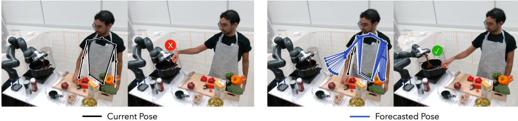
Figure 6: On-Policy Reactive Stirring. (Left) Current: Using the human’s current pose results in a delayed robot reaction and a collision once the human’s hand enters the pot. (Right) Forecast Using the forecasted human position results in a smoother interaction and quicker reaction time, avoiding a collision.
