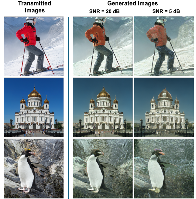
Figure 7. Image reconstructions on unseen DIV2K data. It can be seen that the model does well to mitigate the noise and reconstruct semantically similar images considering that it was not finetuned for this dataset.
