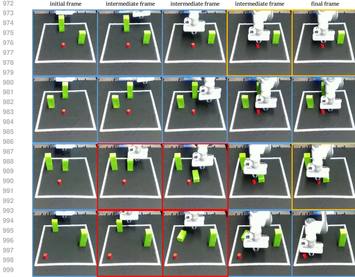
1001 Figure 9. Dataset collection. Each row in the figure represents five frames of the robotic arm’s 1002 motion captured from the same single trajectory. From the moment the robotic arm starts touching 1003 an obstacle to the moment the obstacle’s posture stops changing, the cost label in the dataset is 1004 marked as 1, while in other cases it is marked as 0, as shown in the red-framed part in the image. 1005 When the robotic arm touches the target object, the reward label in the dataset is marked as 1, as 1006 shown in the yellow-framed part in the image.
