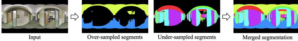
Figure 1: Panoramic segmentation problem can be re-formulated to the estimation of over-sampled segments : floor, ceiling and under-sampled segments : chair, table, bookcase, window, etc.
