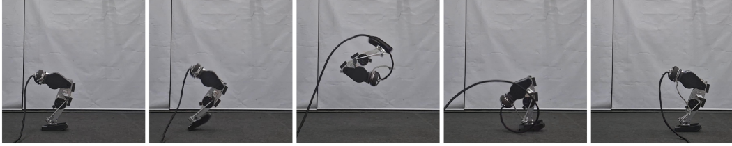
Figure 1: Snapshots of the first successful deployment of the learned front flip on the real one-leg hopper platform. The policy was trained with a centroidal velocity-based reward and sim-to-real techniques to achieve robust, impact-rich rotation on hardware.
