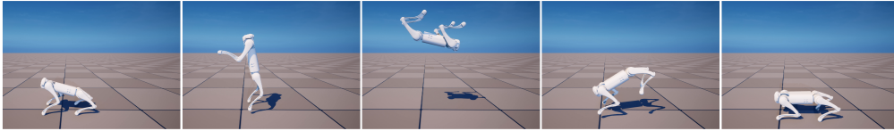
Figure 11: A backflip trained on the Unitree Go1 quadruped.
