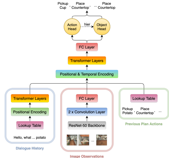
Figure 3: This depicts the architecture for the E.T.-based models. The basic E.T. model does not have a connection between the action and object heads, but E.T. Hierarchical does. There are three main input processing components (dialogue history, image observation, and previous plan actions). These are then input into the positional and temporal encodings and transformer layers to develop the next feasible set of high-level plan actions.
