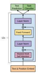
Figure 32: The GPT-2 Architecture. Image from (Radford & Narasimhan, 2018). NanoGPT model is a smaller model with half the number of self-attention layers, multi-heads, and embedding dimensions.
