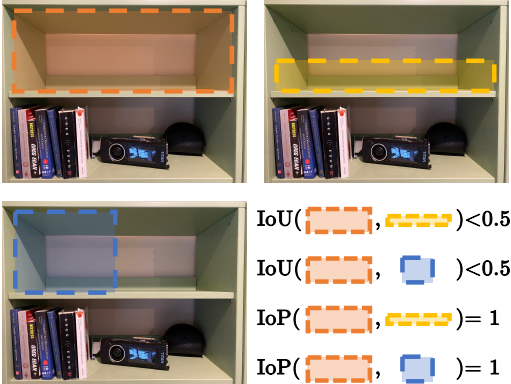
Fig. 6. IoU v.s. IoP. Top left: a hypothetical ground-truth (GT) SP region for objects of type “book”. Top right & bottom left: two possible SP predictions. Both predicted regions are high-quality and should be considered true-positives. The IoU for these predictions is, however, < 0.5 as the IoU normalizes by the large GT region. The IoP, however, only normalizes by the predicted mask’s size and thus is equal to 1 for both predicted regions.
