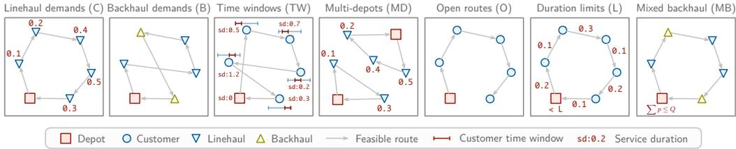
Figure 3.1: VRP attributes. Linehaul demands (C), backhaul demands (B), time windows (TW), and multi-depot (MD) are *node attributes*, whereas open routes (O), duration limits (L), and mixed backhaul (MB) are *global attributes*. Attribute combinations can define new VRP variants.
