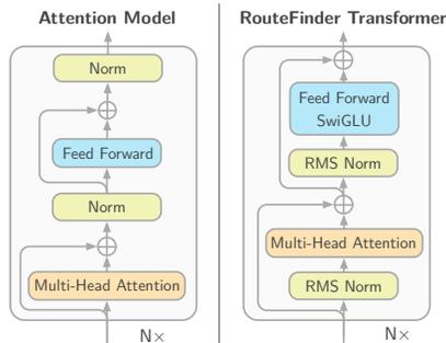
Figure 4.2: Attention model structure v.s. ROUTEFINDER transformer structure.
