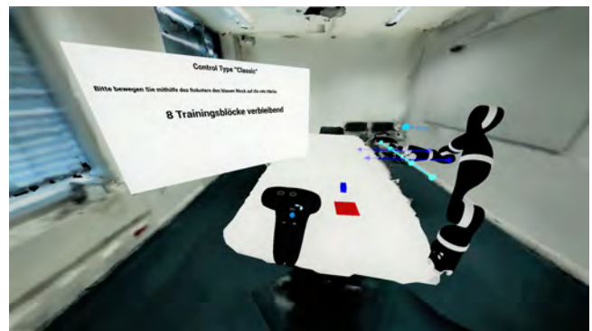
Figure 2: Virtual environment consisting of (left to right): a virtual canvas, the motion controllers, a table with a blue object and red target, and a Kinova JACO with an arrow-based visualization.
