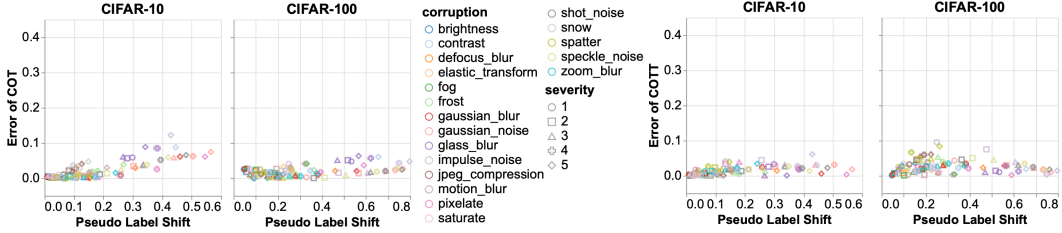
Figure 3: We further compare the sensitivity of COT and COTT’s estimation error to the degree of pseudo-label shift. Compared to Figure 2, we can clearly see that the correlation between the prediction error and pseudo-label shift weakens significantly. Moreover, COTT is even more robust to pseudo-label shift compared to COT.
