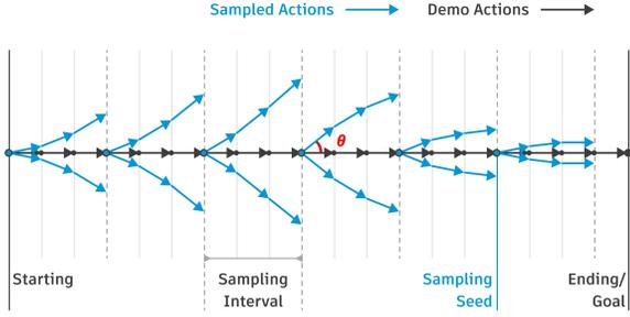
Fig. 2. Temporal variant forward sampling (TVFS). The difference between sampled actions (blue) and demo actions (black) are controlled through  $V(t)$ , which is also a variance measure that changes along the task process.
