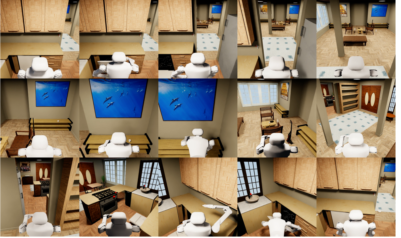
Fig. A.6: Successful task completion by a participant. The robot navigates to a dishwasher and opens it, moves to a table to collect teacups, returns to the dishwasher, places the teacups inside, and closes it.
