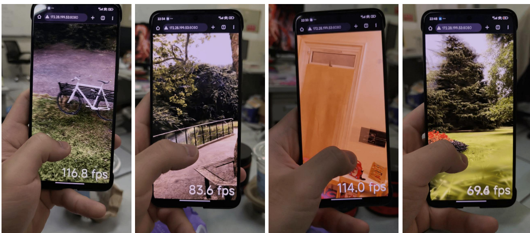
Figure 13: Real-time rendering performance of MEGS 2 on various scenes, showcased via a WebGL-based viewer on Redmi K60 with Qualcomm Snapdragon 8+ Gen 1 . The live frame rate (FPS) for each view is annotated in the imagery.
