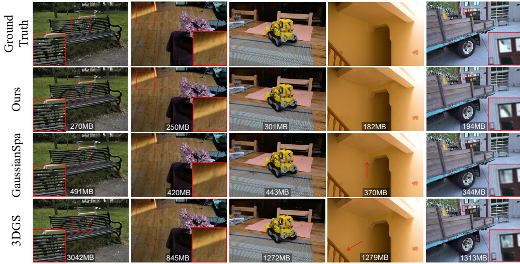
Figure 3: Qualitative results on the Bicycle, Bonsai, Kitchen, Playroom and Truck scenes comparing to previous methods and the corresponding ground truth images from test views. The rendering VRAM consumption for the corresponding method is annotated at the bottom of each image.
