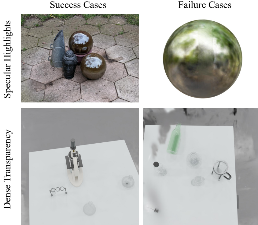
Figure 8: Visualizations of success and failure cases under challenging material conditions. The left column demonstrates successful reconstructions of scenes containing specular highlights and transparency. Conversely, the right column illustrates specific failure cases where we observe reconstruction artifacts under conditions of highly specular highlights or dense transparency.
