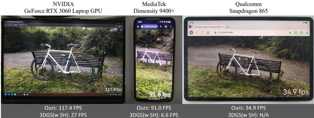
Figure 1: We present MEGS 2 , a memory-efficient framework designed to solve the rendering memory bottleneck of 3D Gaussian Splatting and enable high-quality, real-time rendering on edge devices. As demonstrated in our WebGL-based viewer, 3D Gaussian Splatting(3DGS) with Spherical Harmonics (SH) exhibits low frame rates on desktop GPU and fails to run on some mobile platforms. In contrast, MEGS 2 achieves interactive frame rates across all tested devices, significantly expanding the applicability of 3DGS. The detailed result is in Appendix A.3 and A.4.
