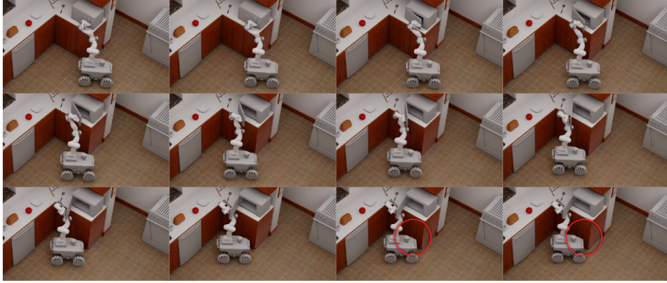
Figure 7: Example of trajectory failure due to collision from simplified robot model.
