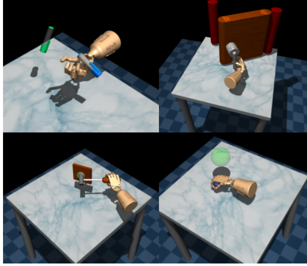
Figure 12: The tasks of Adroit. (top left) Pen - aligning a pen with a target orientation, (top right) Door - opening a door, (bottom left) Hammer - hammering a nail into a board, (bottom right) Relocate - moving a ball to a target position.
