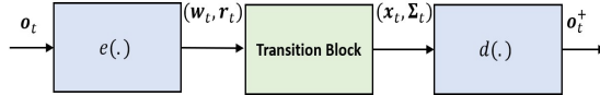
Figure 2: The GIN as a HW model for system identification. By appropriate structure selection for e(\cdot) and d(\cdot) , the GIN can handle high-low dimensional observations. The proposed architectures for each case are depicted separately with further details in appendix figures 10 and 11. The relation between the internal variables, w_t and x_t , is simulated by the transition block.
