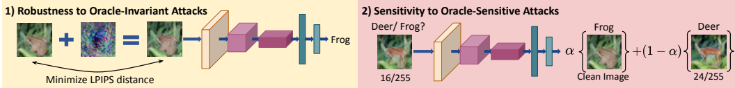
Figure 3: Oracle-Aligned Adversarial Training: The proposed defense OA-AT involves alternate training on Oracle-Invariant and Oracle-Sensitive samples. 1) Oracle-Invariant samples are generated by minimizing the LPIPS distance between the clean and perturbed images in addition to the maximization of the Classification Loss. 2) Oracle-Sensitive samples are trained using a convex combination of the predictions of the clean image and the perturbed image at a larger perturbation bound as reference in the KL divergence loss.
