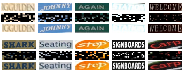
Figure 7: Reconstruction results on images of benchmark datasets (not used in training). For each column, we show the ground truth (top), the masked image (middle), and the reconstructed image (bottom). The visual masking ratio r_v is set to 0.75.
