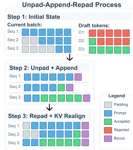
Figure 3: EQSPEC synchronizes via unpad-append-repad.
