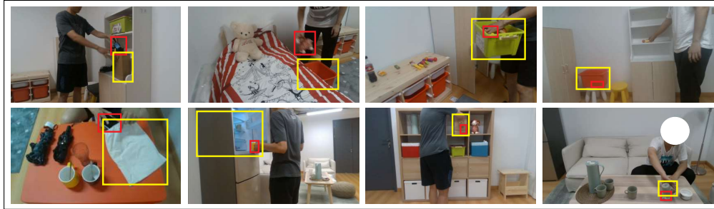
Figure 7: Several tracking examples in the proposed challenging iVOT dataset, where occlusions and containments occur frequently. The red bounding boxes represent the targets while the yellow bounding boxes represent the containers or obstacles.
