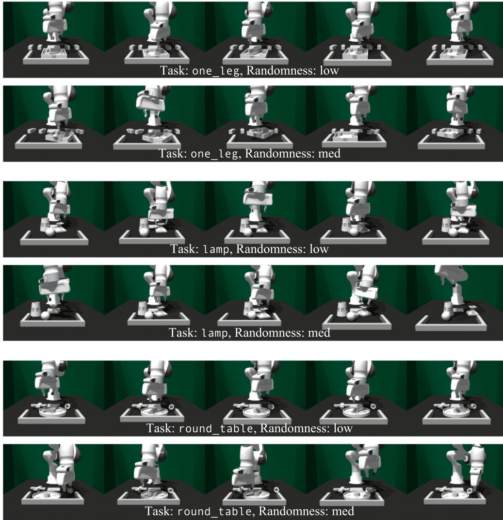
Figure 10: Examples of initial scene layouts for one_leg, 1amp, and round_table with different levels of initial part pose and obstacle fixture randomness
