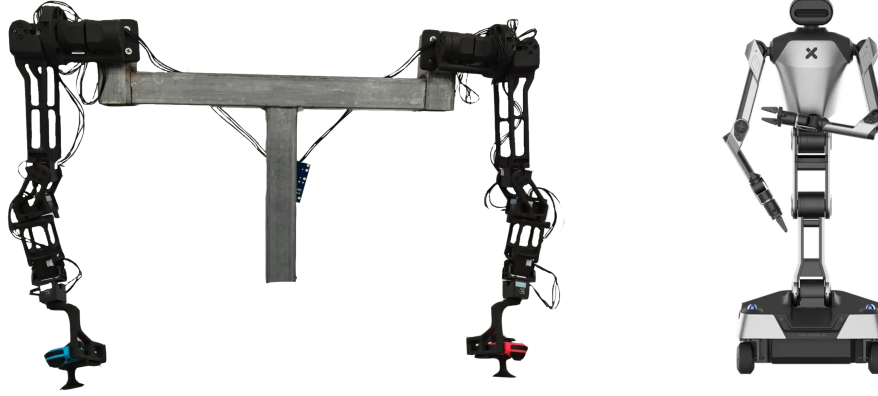
Figure 6: Low-cost JoyLo system and Galaxea R1 robot.
