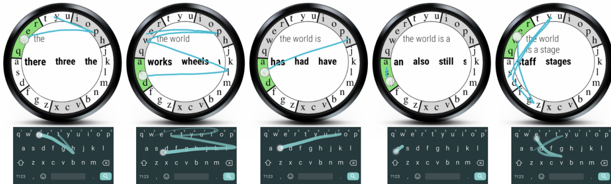
Figure 1: SwipeRing arranges the standard QWERTY layout around the edge of a smartwatch in seven zones. To enter a word, the user connects the zones containing the target letters by drawing gestures on the screen, like gesture typing on a virtual QWERTY. A statistical decoder interprets the input and enters the most probable word. A suggestion bar appears to display other possible words. The user could stroke right or left on the suggestion bar to see additional suggestions. Tapping on a suggestion replaces the last entered word. One-letter and out-of-vocabulary words are entered by repeated strokes from/to the zones containing the target letters, in which case the keyboard first enters the two one-letter words in the English language (see the second last image from the left), then the other letters in the sequence in which they appear in the zones (like multi-tap). Users could also repeatedly tap (instead of stroke) on the zones to enter the letters. The keyboard highlights the zones when the finger enters them and traces all finger movements. This figure illustrates the process of entering the phrase “the world is a stage” on the SwipeRing keyboard (upper sequence) and on a smartphone keyboard (bottom sequence). We can clearly see the resemblance of the gestures.
