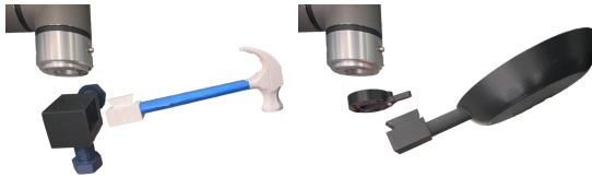
Fig. 12: Fast Tool Changer. Two designs are shown: the left accommodates general tools with a screw mechanism, and the right clips onto tools with specific mounting shapes.
