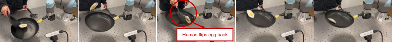
Fig. 6: Human Perturbation Robustness. This figure showcases the robot’s ability to handle human-induced perturbations across three tasks: (1) In nail hammering, the robot successfully followed a manually moved nail; (2) In meatball scooping, it located and scooped meatballs even when additional ones were thrown into the pan mid-task; and (3) In egg flipping, the robot consistently flipped the egg back after human intervention repositioned it. These results highlight the policy’s robustness to unpredictable human perturbations.
