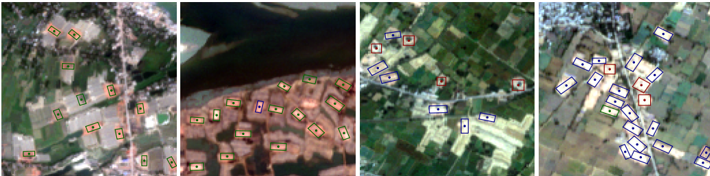
Figure 1: A few samples of Sentinel-2 imagery with Oriented Bounding Boxes (OBBs) around brick kilns. CFCBK (Circular Fixed Chimney Bull's Trench Kiln) is marked in red, FCBK (Fixed Chimney Bull's Trench Kiln) in blue, and Zigzag kilns in green.
