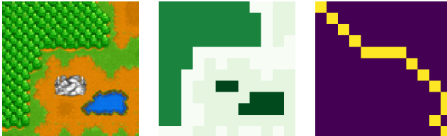
Figure 2: 12 \times 12 Warcraft shortest-path problem. An input terrain map (left), the unsupervised ground truth cost embedding (center) and the ground truth supervised shortest path (right).
