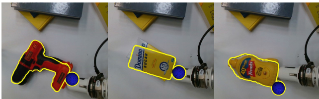
Fig. 5. Results of three example testing trajectory of the physical experiments. The predicted object and robot poses with the optimized \theta highlighted with a yellow silhouette are overlaid with the ground-truth object, robot, and background. [Best viewed in color.]
