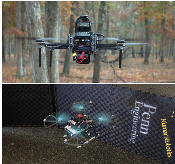
Fig. 1: Platforms used in our deployments. Top : The Falcon 4 has a total weight of 4.2 kg, can fly for more than 30 minutes, and performs autonomous flights greater than 1 km under dense forest canopies. Bottom : the Falcon 250 has a total weight of 1.3 kg and performs missions in indoor cluttered environments. Both platforms run all estimation, path planning, navigation, and control algorithms onboard.
