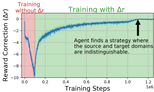
Figure 8: Without the reward correction, the agent takes transitions where the source domain and target domains are dissimilar; after adding the reward correction, the agent’s transitions in the source domain are increasingly likely under the target domain.
