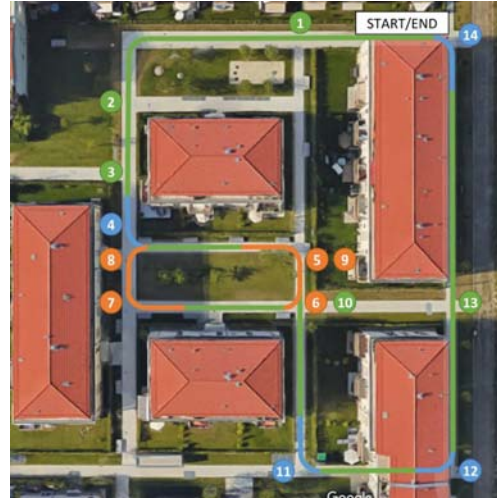
Fig. 8. A map of the primary route used for testing the physical system. Intersections traversed by the truck are numbered according to their order along the route. Colors indicate commands provided to the vehicle when it approaches the intersection: blue = left, green = straight, orange = right.
