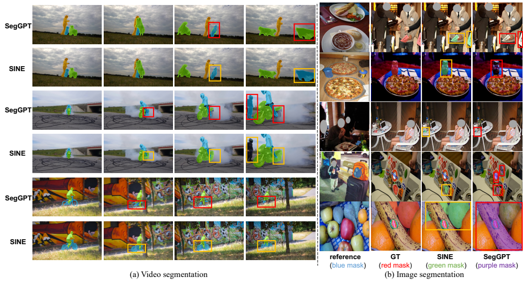
Figure 7 – Visualization comparisons between SINE and SegGPT on video and image tasks. For video task, SINE can effectively alleviate the tracking failure issues caused by crossing, perspective changes, occlusion, etc. In real-world image segmentation, SINE has a stronger category generalization capability compared to SegGPT and can effectively alleviate the ambiguity problem.
