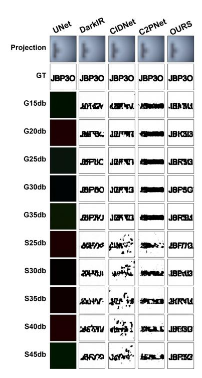
Figure 18: The noise experiment results on the Resh-screen dataset. Each row corresponds to a model; the first column shows the projected image, the second column shows the ground truth (GT), and the subsequent columns represent the model's performance under different types and levels of injected noise, where G denotes Gaussian noise and S denotes salt-and-pepper noise.
