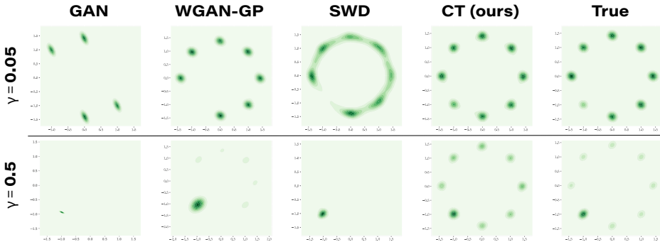
Figure 3: Experiments on the resistance to model collapse: Comparison of the generation quality on 8-Gaussian mixture data: one of the 8 modes has weight \gamma and the rest modes have equal weight as \frac{1-\gamma}{7} .
