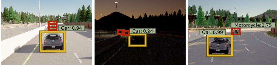
Figure 4: Left to Right: misdetection due to Mode 1 (distance), Mode 2 (poor light) and Mode 1 and 2 (distance and poor light), respectively. Bounding boxes for detected objects (misdetections) shown in yellow (red) with detection confidence numbers. Each scene has two cars and a pedestrian.
